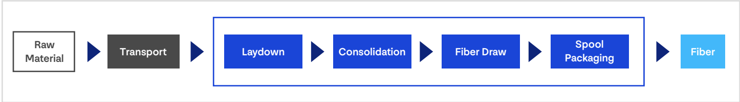
Figure 5: Manufacturing Process Flow of the Optical Fiber
